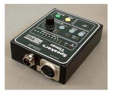
An external plug pack connects via a 2 pin locking metal connector. The plug pack can be 16-18V AC 1 amp or 24V DC at 500mA. The connector can be wired with either polarity as there is an internal rectifier. A suitable plug pack is supplied.
