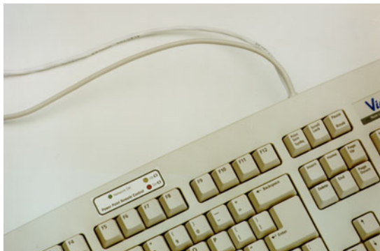
Modified keyboard showing additional LEDs and cable.
